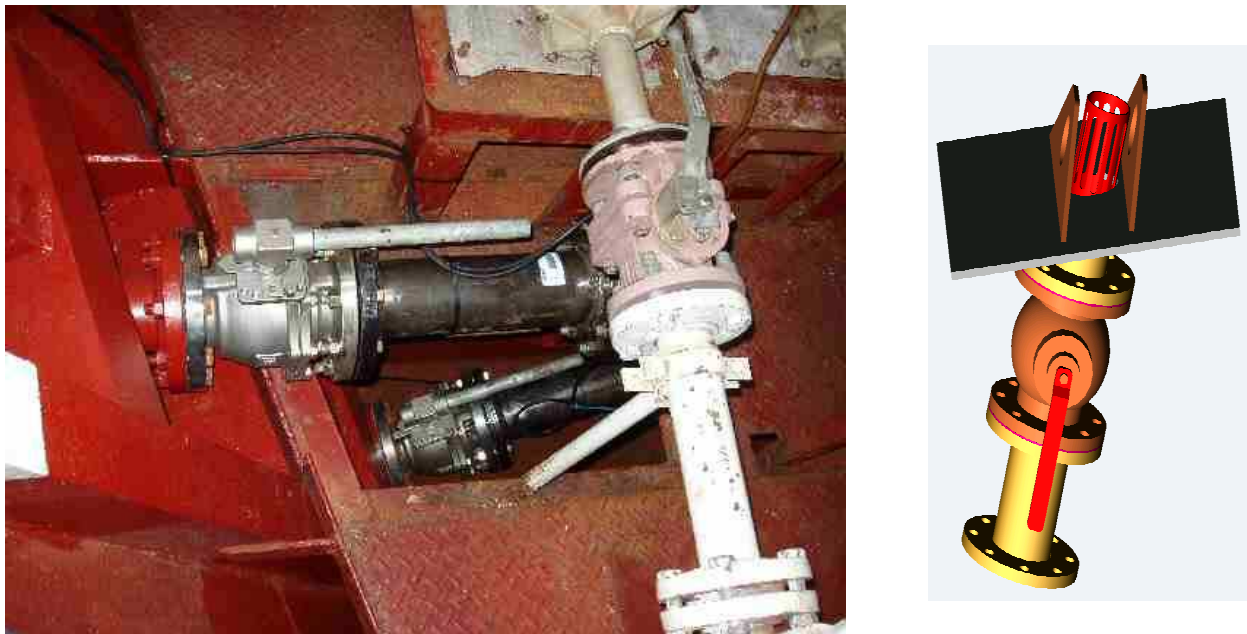
Figure 3. Through-the-hull sensor ports located in the bow thruster room on the Brown . The ports are 2 m and 3 m below the water line.
